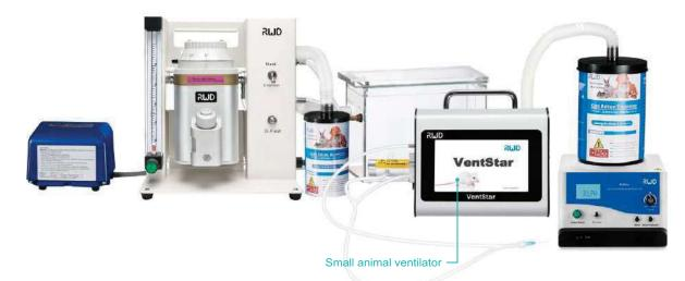
This program is the combination of anesthesia machine and ventilator. While keeping the animal under anesthesia, it provides a certain volume (tidal volume) of oxygen and respiratory rate to support the normal breathing of animals.
