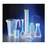
PMP: Polymethylpentene; can be autoclaved to 121ºC without affecting the graduation tolerance
