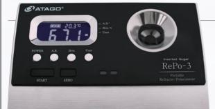
Inverted Sugar is a sweetener made by hydrolyzing (splitting) sucrose into glucose and fructose. In contrast to sucrose and glucose, which exhibit slight dextrorotation, fructose has strong levorotation. This instrument displays the amount of sucrose that was converted as an inverted ratio (%).
