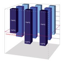
Comparison of temperature distribution in a liquid nitrogen freezer (vapour phase) and our MDF-C2156VAN mechanically refrigerated **Cryo**genic Freezer. The graph shows temperatures at different locations within the chamber
