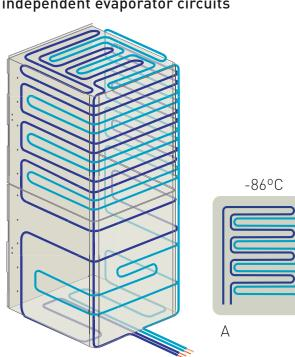
• The Dual Cooling System offers the highest level of security through the use of two independent refrigeration systems. If one system unexpectedly fails the other can maintain the freezer at the -70°C range.
