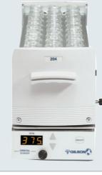
The Orbital Shaker is specifically designed for on-line or off-line liquid handling, vortexing, and mixing. It is a fully functional, stand-alone instrument. This compact shaker fits on one rack position of a GX-281 Liquid Handler bed. The shaker provides a range of customer-controlled shaking (20 to 720 rpm), allowing vortexing on various vessel sizes and sample volumes.
