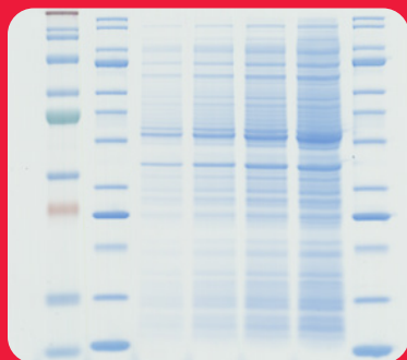
12% TurboMix™ Bis-Tris hand-cast gel loaded with E. coli lysate titrations (lanes 3–6), mPAGE® unstained protein standard (lanes 2 and 7), and mPAGE® color protein standard (lane 1). Gel was run with MOPS buffer for 35 min at 200 V and stained with ReadyBlue™ Protein Gel Stain.
