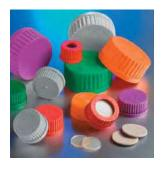
Caution: Bottles larger than 2L should NOT be used with bottle top filter units, or in other applications involving vacuum pressure, as breakage may occur. DO NOT have caps tightened immediately after autoclaving, as the vacuum resulting from cooling can cause breakage. A pouring ring is not included on 25 mL size. A vented cap is NOT recommended for use on the 5L and 10L 1395 series bottle.
