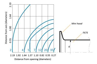
Figure 6.2 shows the capture zones at two different airflows. The capture zone is defined for the conditions; extract 97% of the contaminant with 0.25 m/s horizontal cross-draught. The test is made with FX75 with mini hood positioned sideways over a table.
