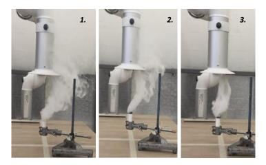
The tests are made for three different capture hood positions to investigate how this affects the capture rate. The hood positions are shown in figure 3.2 and called *above*, 45° and *sideways*. In the following diagrams their test values will be shown with the color of each frame below.
