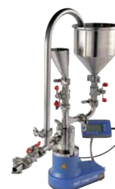
magic LAB® with module CMS and accessories for powder incorporation into liquid in recirculation mode
