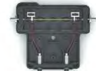
Max-Light cartridge cell, interior view, 60 mm path for high concentrations, G4212-60007
