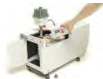
Adding foreline pump (rotary pump) oil, 4 L
