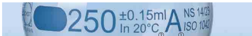
Tolerance indication with a volumetric flask in accuracy class A (1) with a tolerance of \pm 0.15 ml (2)
