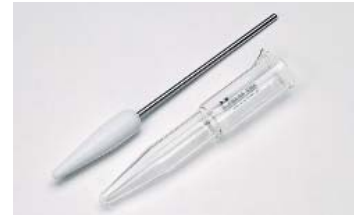
Homogeniser with overflow flare with lip and teflon pestle, tapered
