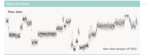
As a DNA or RNA strand passes through the nanopore, the current is measured several thousand times per second. These current samples are known as raw data, which is subsequently processed using machine learning techniques into basecalled data — the sequence of DNA or RNA bases
