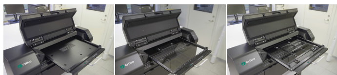
Fig 4. (A) The IP stage, (B) fluor stage, and (C) multi-stage are designed to accommodate a variety of sample formats and imaging modes.
