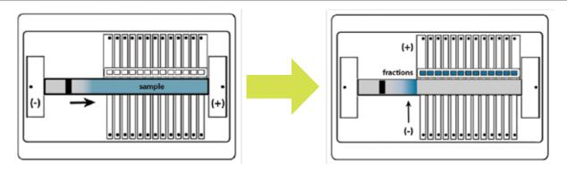
The SageELF gel cassette separates DNA along an agarose gel column. At the end of a user-programmed run time, a second set of electrodes is activated. DNA fractions are then side-eluted into 12 membrane-bound wells. The cassette design includes a novel continuous buffering system which ensures DNA does not diffuse away from the gel during separation, and that fractions are evenly collected during electro-elution.
