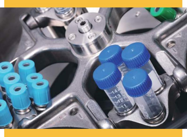
The centrifuge used to separate liquid and solid particles or components in a liquid mixture. The DLAB centrifuge series includes palm micro centrifuges, high-speed centrifuges (refrigerated and non-refrigerated), hematocrit centrifuges and low-speed centrifuges.
