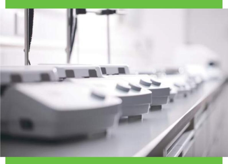
Magnetic hotplate stirrers are used for low viscosity liquids or solid mixing, widely used in chemical synthesis, physical and chemical analysis, bio-pharmaceuticals etc. DLAB provides different series, heating range covers from 120°C-550°C:
