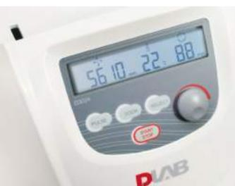
Speed/RCF switch; Short-time run function; sound-alert function
