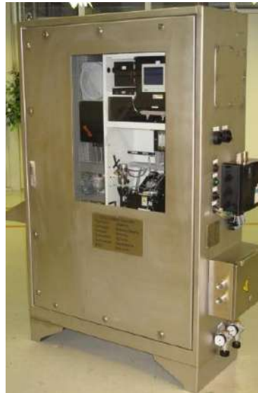
Fig.: TOC analyser in pressurized cabinet
