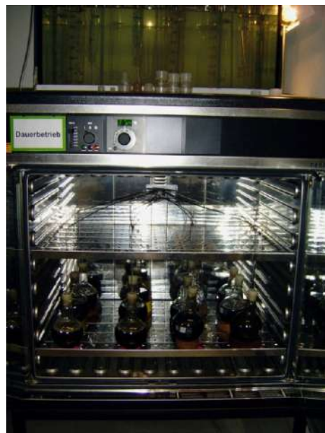
Fig. Experimental setup to generate bio gas in the laboratory
