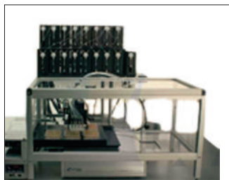
Figure 3. The CrystalScore system is an automated imager that has a motorized x-y stage that automatically moves to each well and captures an image with a high-resolution digital camera.
