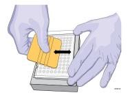
**3.** Rub the flat edge of the applicator back and forth along the short edge (width) of the plate.
