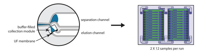
Sage Science's proprietary technology, featuring electro-elution from agarose, has been configured to run 12 samples on an SBS-footprint gel cassette— *for higher-throughput workflows and with a lower cost per sample.*
