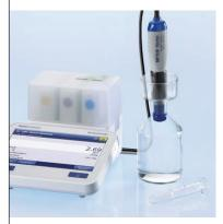
The BOD content of any effluent can be checked very easily. With the special BOD adapter, the sensor is suitable for measuring in all current types of BOD bottles. According to the EPA (Environmental Protection Agency, USA), stirring is not necessary thanks to RDO technology. With the S900-BOD Kit you are ready to start.
