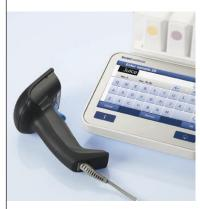
The instrument's touch screen operation makes the entry of text, e.g. sample ID's, possible in a quick and convenient way. To even further increase efficiency, you can use a USB barcode reader.
