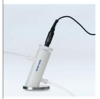
Low conductivity measurement requires special attention. When measuring pure or ultra-pure water there are several sources of potential error such as carbon dioxide from air and temperature inaccuracy. Our digital conductivity cell InLab® Trace, with high temperature accuracy and optional flow through cell now provides the perfect solution.
