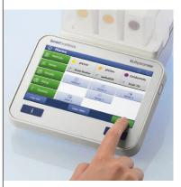
This instrument encompasses a second possibility to start a measurement or calibration by pressing READ or CAL. Although more flexible, performing direct measurements in a row with varying parameters requires a change of settings before each sample.
