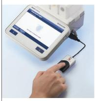
In addition to typing a password, the instrument also supports the LogStraight™ external fingerprint reader. This not only offers a convenient login solution, but also provides an extra degree of security!
