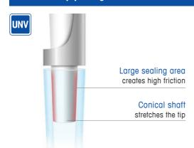
Universal pipettes have cone-shaped shafts that rely on friction to hold tips firmly.
