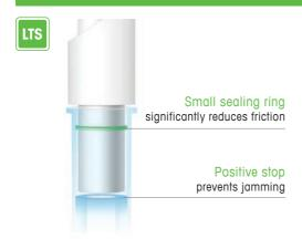
The Rainin LiteTouch System dramatically reduces the amount of force required to load and eject tips. LTS pipettes work in concert with LTS tips to deliver a perfect seal every time.
