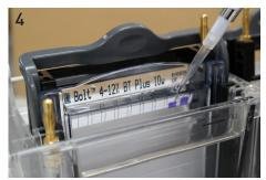
**4.** Make sure the wells are completely filled with 1X buffer.
