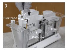
**3.** Make sure any cassette clamps are removed from the chambers.
