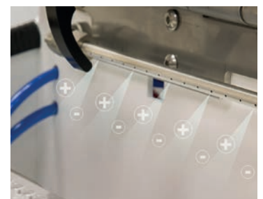
Ionizer bar to combat static electricity
