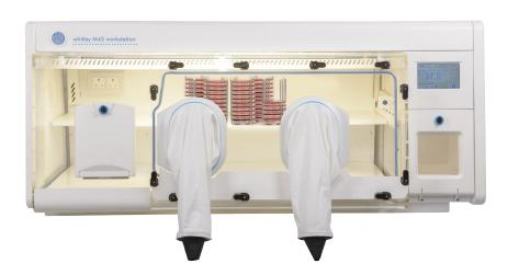
The M45 has three ports for convenient user access to the entire incubation and working areas. This workstation can accommodate over 780 x 90mm Petri dishes whilst still providing a generous working area. The M45 is used in the study and isolation of fastidious anaerobes such as *Campylobacter* spp. and *Helicobacter pylori*.
