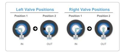
**Note:** The left and right valves can move independently of each other, as indicted in the diagram above.
