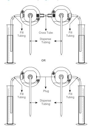
In a dispensing application there are two configurations possible. Use the top configuration if you plan to switch between diluting and dispensing applications. Use the bottom configuration if you are only dispensing and are concerned about sample carryover.
