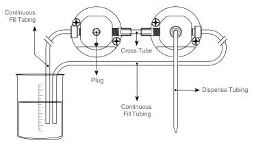
Note: All dual syringe pumps will come from the factory set in the diluter configuration. If this is not the desired application, refer to the appropriate configuration and change the pump accordingly.
