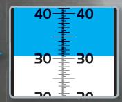
Read the measurement value where the boundary line intersects the scale.
