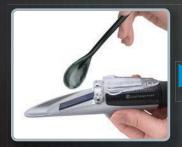
1 Apply 1-2 drops onto the prism.
