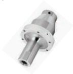
Booster horns increase the intensity of standard ¾" and 1" horns. Boosters attach between the converter and horn to increase amplitude by the gain ratio indicated below.
