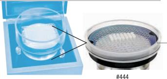
The Microplate Horn is commonly used in PMCA research. A microcentrifuge tube holder and cover (#444) are available and often used for this application.
