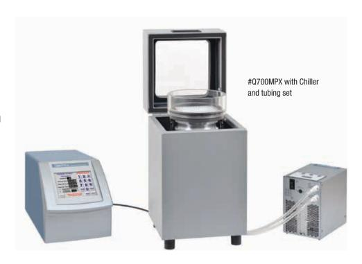
The Horn is equipped with a clear acrylic collar to contain the liquid media within the reservoir. This allows the user to process deep well microplates or other tall vessels. Standard microtiter plates or PCR tubes require a smaller volume of liquid for sonication. For these applications, the clear acrylic collar may be removed and the lower, gray collar will allow for easier access to the samples.
