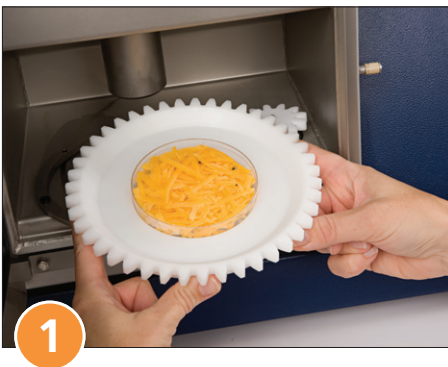
1 Fill up the sample cup and place it in the instrument
