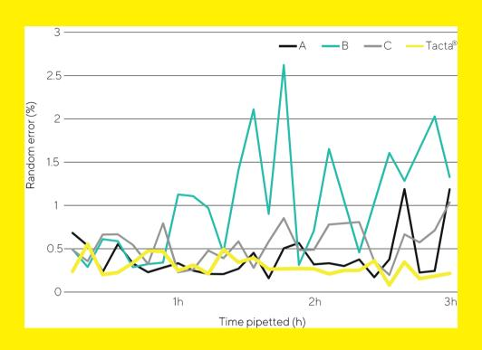
Precision of results tested over a three-hour period using four pipettes from various manufacturers. The test was performed by an independent laboratory in accordance with the ISO 8655 standard using 1000  $\mu l$  pipettes with 1000  $\mu l$  tips from the corresponding manufacturers.
