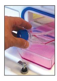
Introduce individual samples without compromising internal atmospheric conditions
