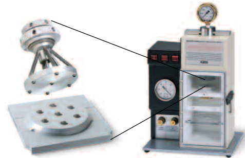
The PDS-1000/He system, shown here with magnified view of the Hepta adaptor.
