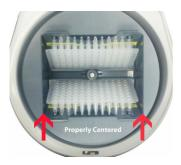
**Figure 1** Example of Properly Balanced Rotor
