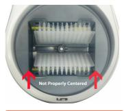
**Figure 2** Example of Improperly Balanced Rotor
