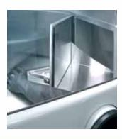
The Biowizard BW-3 is a Class III safety cabinet which protects the operator and the environment from hazards in handling infected and other dangerous biological material.
