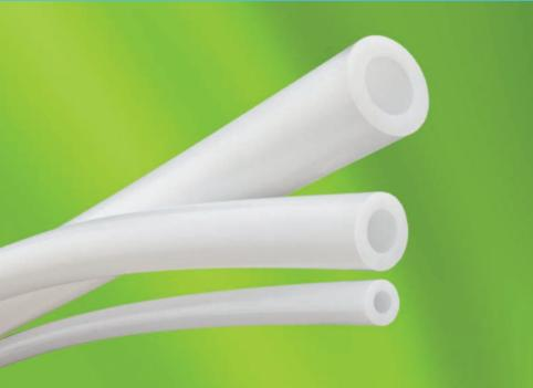
PTFE-reinforced silicone tubing which provides long term performance with repeatable accuracy, vital in pharmaceuticals and other high technology industries. Suitable for pressures up to 7 bar (100 psi), GORE STA-PURE PCS provides the longest available tube life with virtually no spallation.
